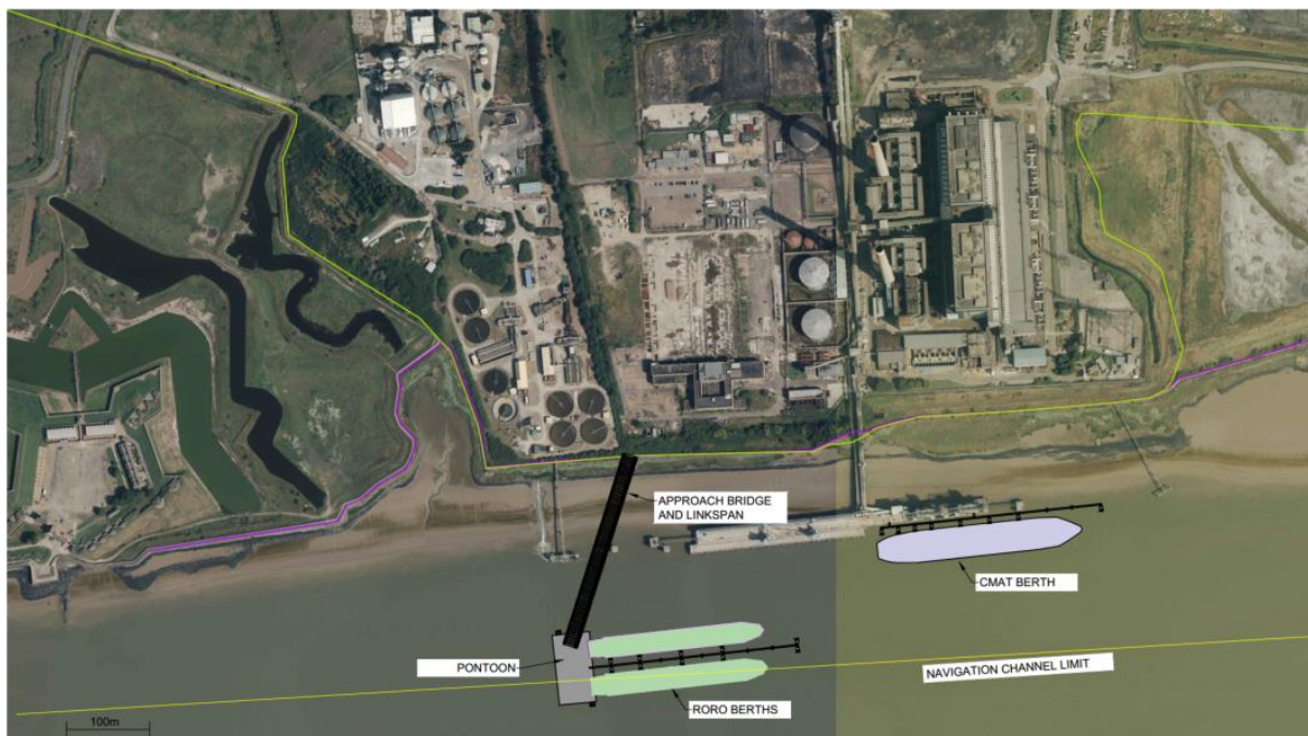
Figure 2: Side by Side Ro-Ro berth
